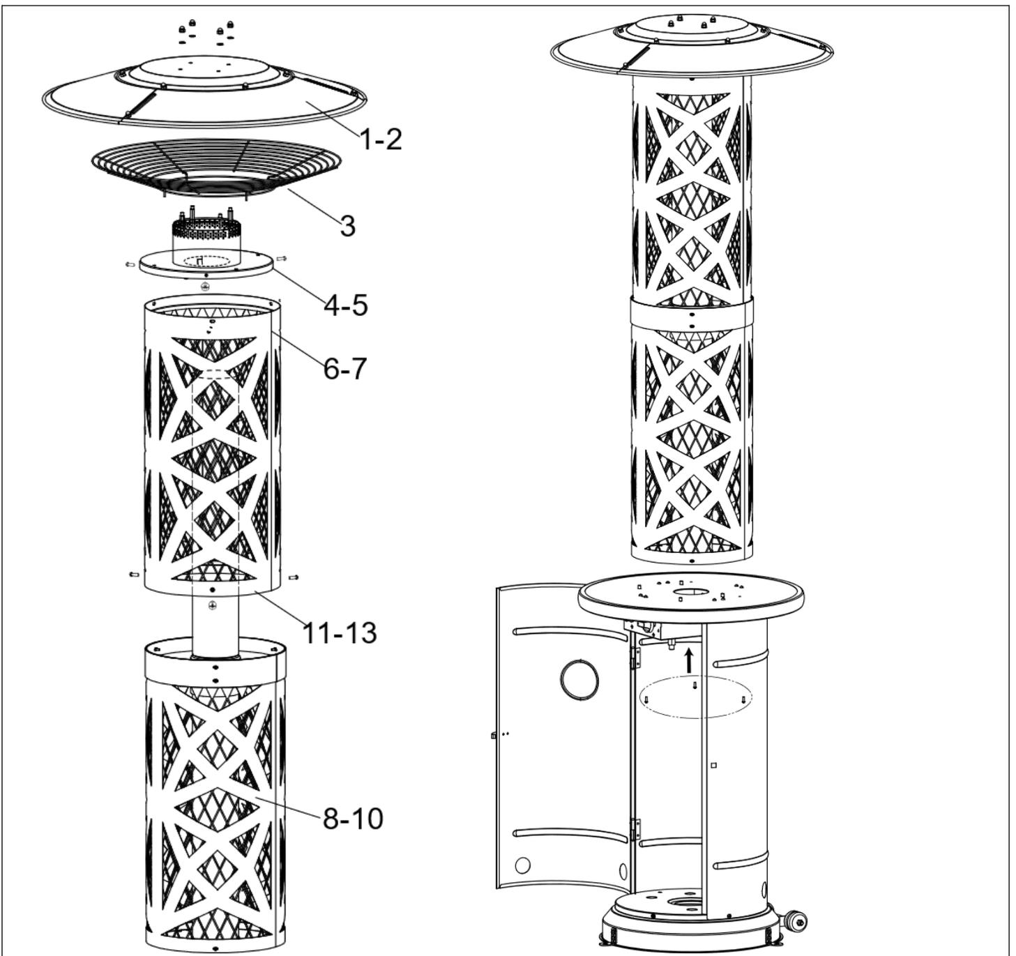
**STEP 7:** Place assembled Decorative cover (6-7), Flame screen with supports (4-5), Protection grid (3) in order, then fix these parts using 6pcs M4x12 screws (GG).
