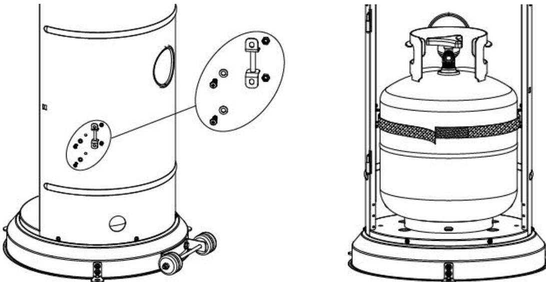
5. Fix both velcro tapes onto rear of tank housing using preassembled 4pcs M5\*12 screws,  $\Phi 5$  washer, M5 nuts.
