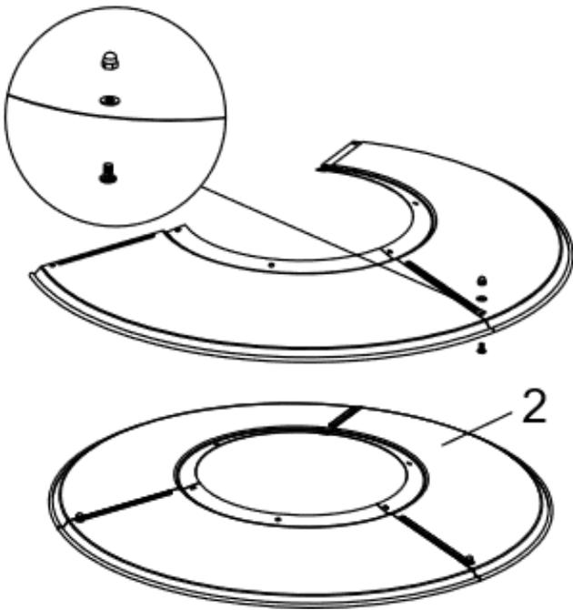
**STEP 5:** Attach Reflector plate (2) together using 3pcs M6 x 8mm screws (BB),  $\Phi 6$  washers (CC) and cap nuts (AA). Secure loosely with cap nuts.
