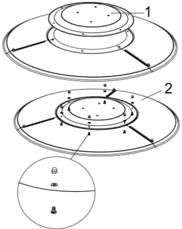
**STEP 6:** Attach Reflector plate (1) to Reflector dome (1) using 6pcs M6 x 8mm screws (BB),  $\Phi 6$  washers (CC) and cap nuts (AA). Secure loosely with cap nuts.
