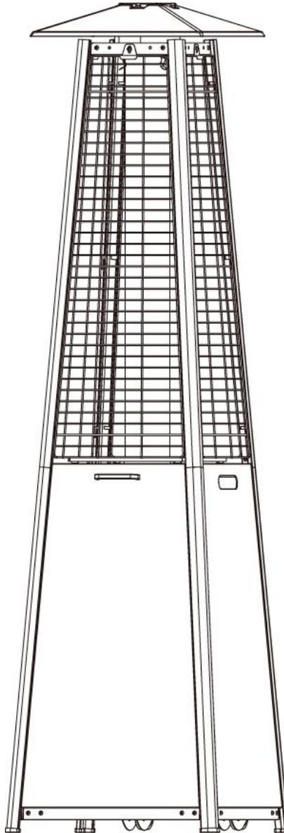
This model flame heater height is 1.9m and the base is powder coated steel
