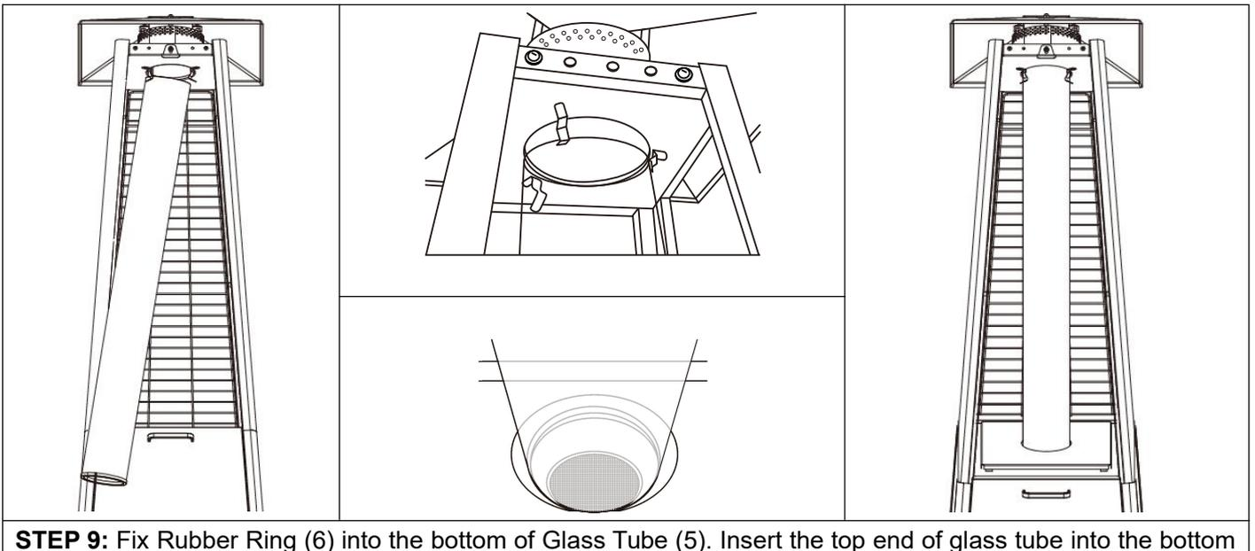
hole of Flame Screen (2) as much as possible. Keep glass tube vertically and sit it in the hole of Plate Cover (8).
