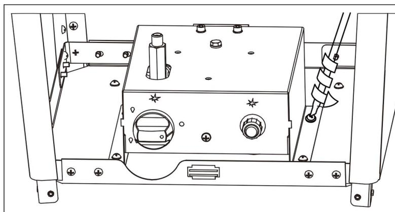
**STEP 2:** Lay down tank housing, fix the Burner Assembly (9) to Pate Cover (8) by 4pcs M5 Screws and Washers (BB).
