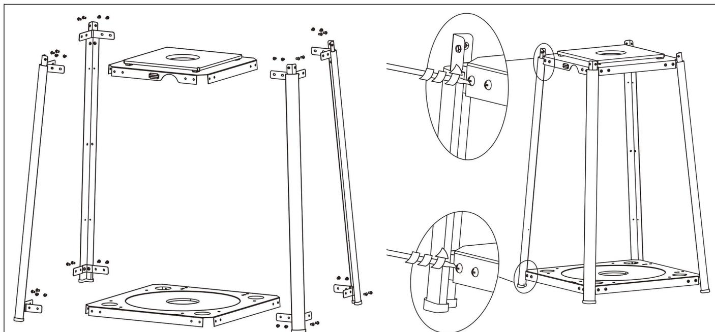
STEP1: Connect and fix the 4 Support Bar – Lower (1) to Bottom Plate (14) and Plate Cover (8) by 32PCS M5 screws and washers(BB)
