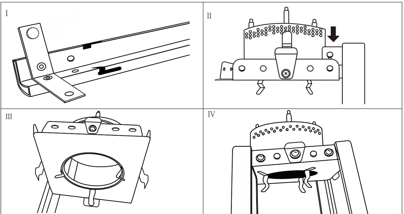
**STEP 5:** Attach Flame Screen (2) to the top of Support Bar-Upper (3) and fix the connection with 2pcs M5 screws and washers (BB), (See Figure I , II).
