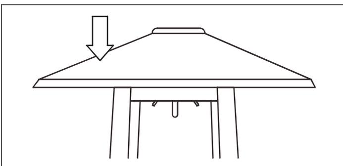
**STEP 6:** Place Reflector (1) on the Flame Screen (2) and fix the connection with 4pcs M5 CAP NUT (AA).
